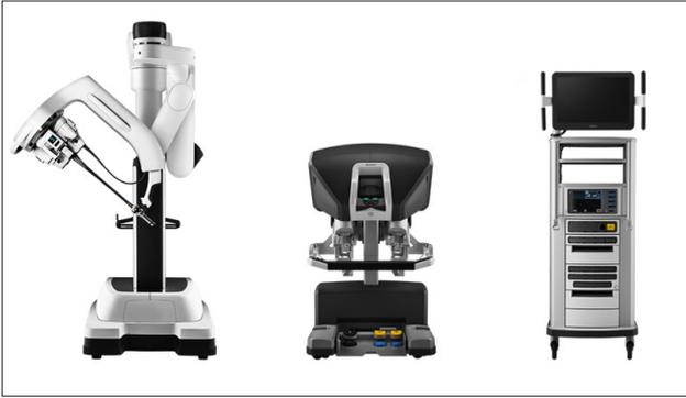
**Fig. 1.** Da Vinci single port (SP) system. The system includes the patient-side cart (A), surgeon's console (B), and the vision cart (C). Adapted from Intuitive da Vinci<sup>12)</sup> with permission of Intuitive.
