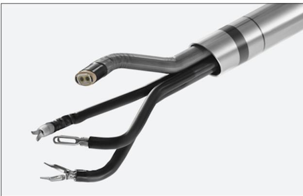
**Fig. 2.** Instruments of the single port (SP). A multi-articulating camera and three double-jointed articulating endowristed instruments within one cannula eliminates external arm collisions. Adapted from Intuitive da Vinci<sup>12)</sup> with permission of Intuitive.
